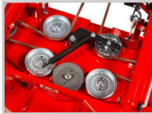
Deck drive belt system is designed to provide even belt tension which improves the life of the belt and reduces maintenance.
